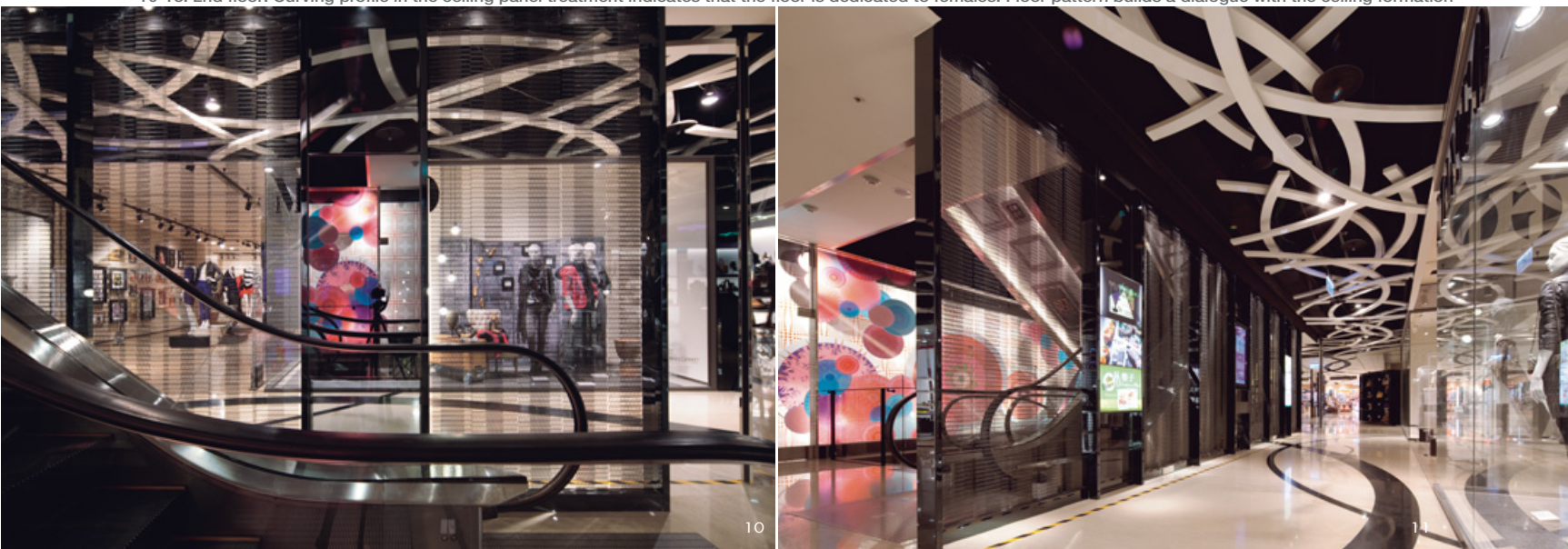
10-13. 2樓，天花板採用白色金屬烤漆的雙環結構呼應女性商品的柔性感，環狀線條亦輔助動線引導。手扶梯立面為半穿透的輸送網，地面以深色勾線呼應天花板的環狀造型。 10-13. 2nd floor: Curving profile in the ceiling panel treatment indicates that the floor is dedicated to females. Floor pattern builds a dialogue with the ceiling formation
